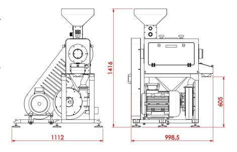
The machine is equipped with a charge hopper that regulates the product's flow. The outlet is equipped with an adjustable device which allows to regulate the staying time of the kernels inside the machine and, consequently, their husking degree.
